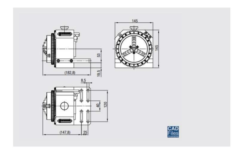
Plan drawing of direct dividing head VA with three-jaw chuck DBF 100
